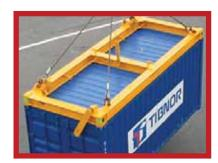
Timars HCL spreader is a rectangular shaped frame container spreader for handling ISO certified containers. The spreaders design will sustain extremely rough conditions.
