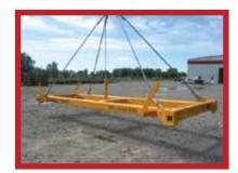
Timars HCA Spreader is a low cost no frills spreader that can be supplied in three pieces and then bolted together at destination. This makes it easy to ship as LCL cargo in standard containers that reduces the landed cost significantly.
