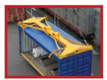
Timars C-Lift spreader is a flexible fixed frame spreader for handling of ISO containers. The spreader has a very low tare weight, which makes it perfect for ships and smaller cranes. The spreader is designed to withstand tough climatic conditions and harsh marine environments.
